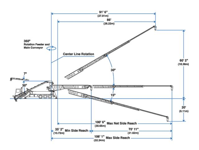
The TB 110 can place concrete at high volumes up to 360 yd³/hr (275m³/hr) and convey a wide variety of materials ranging from sand to 4" (100mm) rock. With its steel/aluminum truss and three aluminum sections, this four-section telescopic conveyor offers 106' 1" (32.34m) of horizontal reach. The unit can set up and operate under heights as low as 15' 9" (4.80m).
