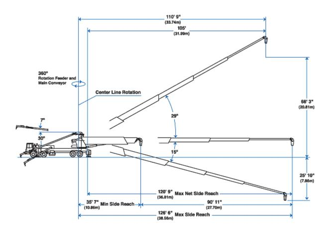
Offering a 126' 6" (38.56m) horizontal reach, the TB 130 features a five-section boom and a fully hydraulic conveyor capable of handling concrete slumps from 0" to 12" (0mm to 305mm) and materials from sand to 4" (100mm) rock. Strong yet lightweight and easy to control, the unit features quick setup using its patented outrigger design. The TB 130 also operates in ceiling heights as low as 15' 4" (4.70m).
